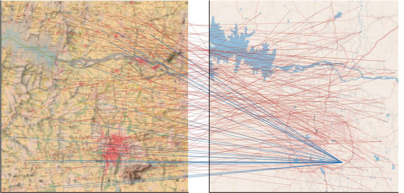
Figure 3: Correspondences between the 1926 scan (left) and the OSM render (right). Blue: RANSAC inliers. Red: a sample of rejected matches. (a) LoFTR’s inliers agree on one transform and cluster along the Cauvery corridor and the railways. (b) SIFT’s 594 ratio-test matches support no consistent model. The 26 “inliers” of the model MAGSAC++ returned collapse onto a single point of the reference, the degenerate solution that the validity checks reject.
